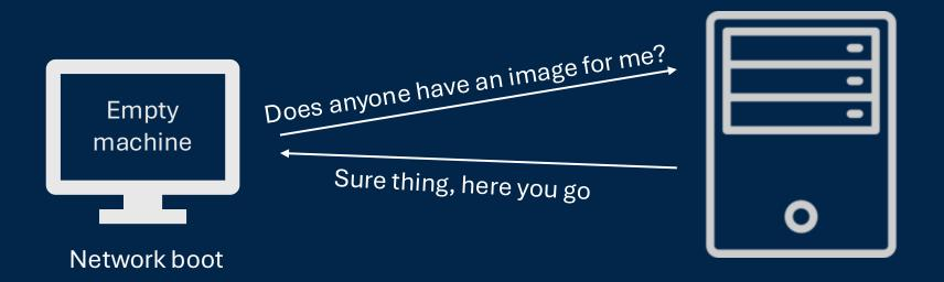
Images are downloaded over the *Trivial* File Transfer Protocol (TFTP) No encryption, no authentication
